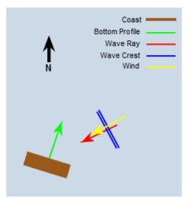
Figure B.8 Orientation of the bottom profile, wave- and wind direction with respect to the coast (Source: own illustration)
