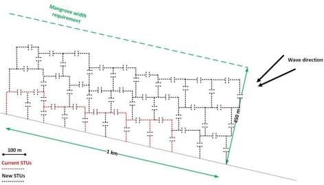
Figure 6.7 Phase 2 of construction STUs after required sedimentation in phase 1 is reached (Source: own illustration)
