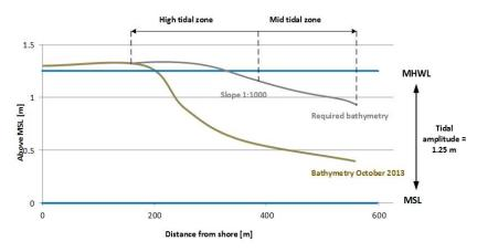
Figure 4.14 Current bathymetry and required bed level (Source: own illustration)
