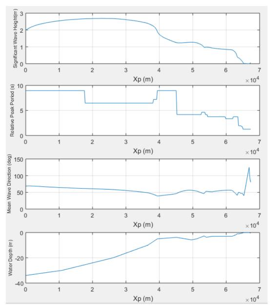
Figure B.14 Results SwanOne for swell waves (Source: own illustration)
