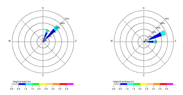
Figure B.1 Direction and height of swell and wind waves during Summer (July-September) (Source: BMT ARGOSS, 2017).
