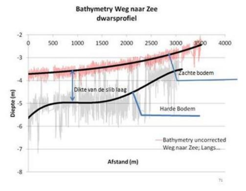
Figure 2.4 Thickness soft mud layer (Source: Naipal, 2013)
