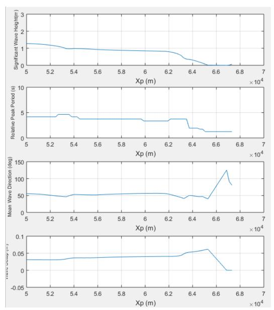
Figure B.15 Results SwanOne for swell waves (Source: own illustration)
