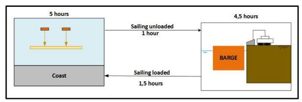
Figure 6.24 Total cycle time of the construction of the chenier (Source: own illustration)
