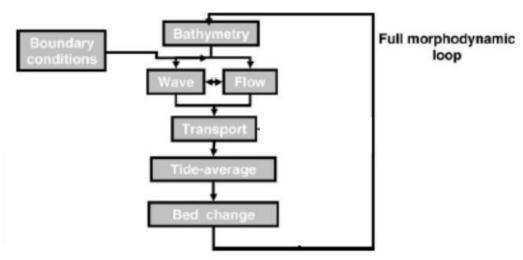
Figure 6.25 Morphodynamic loop in the Delft3D model, (Source: Walstra, 2017)
