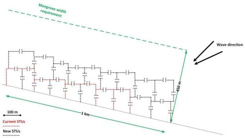
Figure 6.6 Phase 1 of construction STUs after required sedimentation in phase 0 is reached (Source: own illustration)
