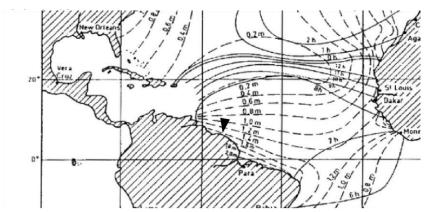
Figure 2.9 Tidal propagation in front of the coast of Paramaribo (Bosboom et al.,2015)
