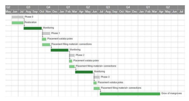
Figure 6.13 Gantt Chart of the construction for Preliminary design 1 (Source: own illustration)
