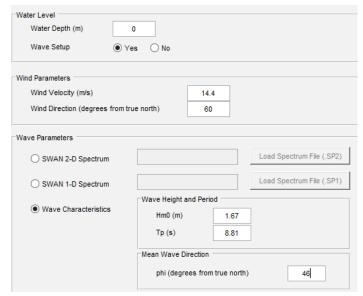
Figure B.11 Input parameters in SwanOne (Source: own illustration)
