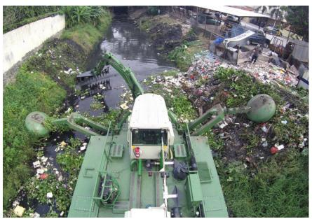
Figure 6.21 Cleaning of a channel with the amphibious vehicle of Watermaster (Source: Watermaster, n.d.)
