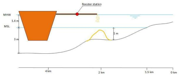
Figure 6.23 Construction method, placing of the chenier (Source: own illustration)
